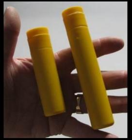
These cartridges contain their own firing pins and initiation primers. The cartridges are activated by the impulse (shock wave) traveling down the column of water. The maximum distance from the tool to the top cartridge should not exceed one meter. In deeper holes, use the cartridge wings to strategically place and space the cartridges.
