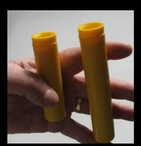
This picture shows the tops of the power cartridges. They should be placed in the drill hole with the top end up, (facing the tool)
